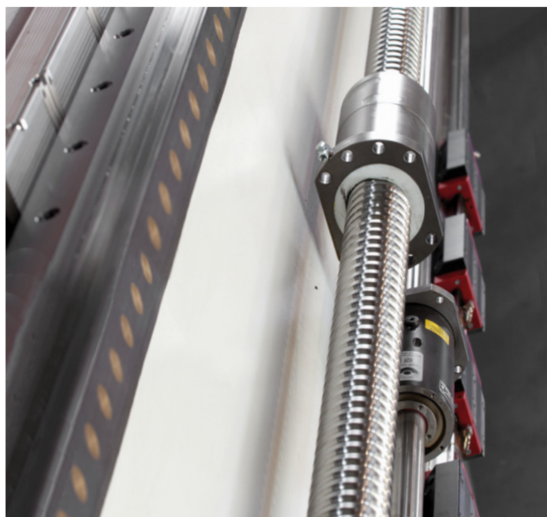
Compact guide ways, ball screws and a direct measurement system
