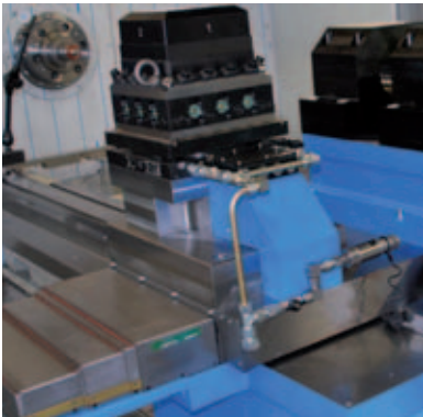
Clamping bearing for boring bars with changeable bearing inserts for different diameters. 2 clamping points and additional guiding on the bed slide. Installed behind the turning center.
