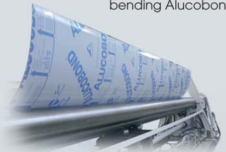
Special "soft materials" machine for example bending Alucobond®.
