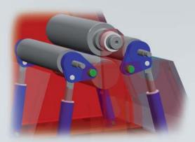
This technology nearly eliminates the slipping sliding friction for side rolls movement.
