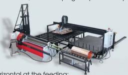
horizontal at the feeding: The possibility to use the optionals gantry loader and an in-feed conveyor (together with the HI-TECH DAVI's CNC) makes the MCA the best solution to improve productivity, by shortening the cycle time and reducing the hand work needed for the plate handling.
