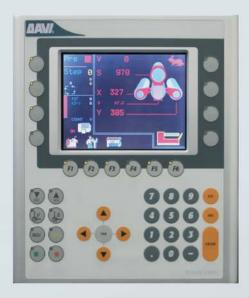
Recommended to users that need to program as simple as possible single radius parts. This innovative CNC, thanks to its powerful Intel Pentium<sup>®</sup> processor, is selfprogramming, complete automatically, through the "Computer Program Mode" any single radius shape (the multi radii parts can be programmed Teach-in or in Editor mode).
